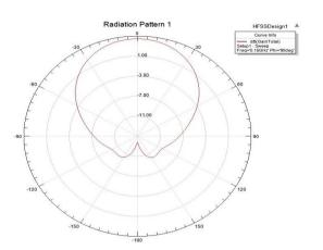
Figure 5: Gain pattern at 150MHz
